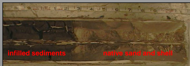
Stratigraphic cross-section from vibracores collected along a transect normal to the channel.
